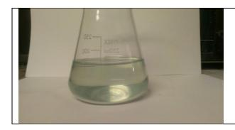
A chrome (vi) solution after the titration with 0.1M sodium thiosulphate.
